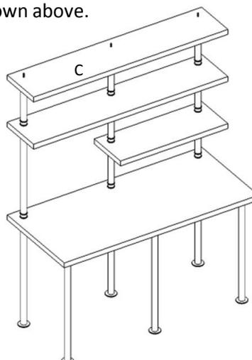
STEP 8 - Insert a Long Shelf (C) onto the Solid Rod (E) as shown above.
