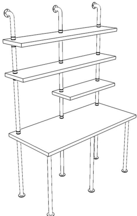
To complete the installation fix the unit to wall with the screws (1) and Plastic Anchors in the predrilled holes in Bent Pipe (A) as shown above.
