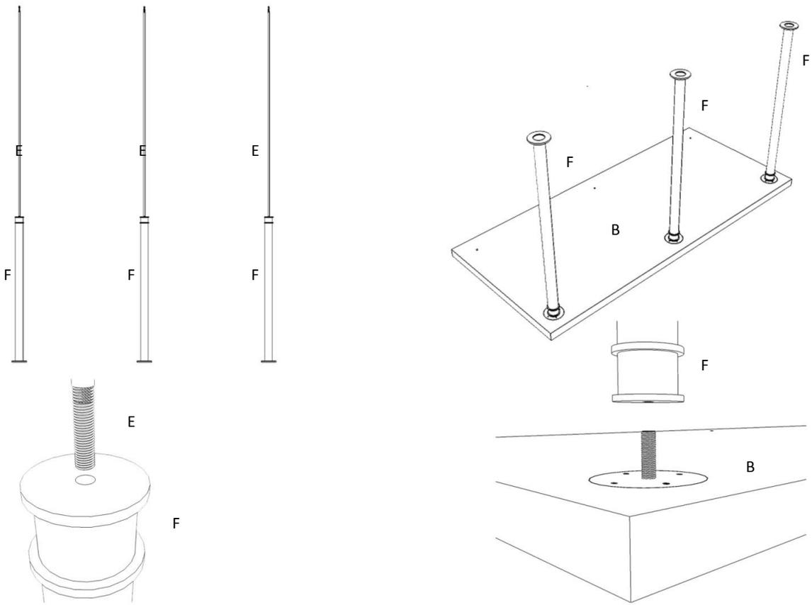
**STEP 1 – Attach Bottom Leg (F) to Solid Rod (E) to make the support rod. Attach remaining 3 pcs of Bottom Leg (F) to Table Top (B) as Shown Above.**
