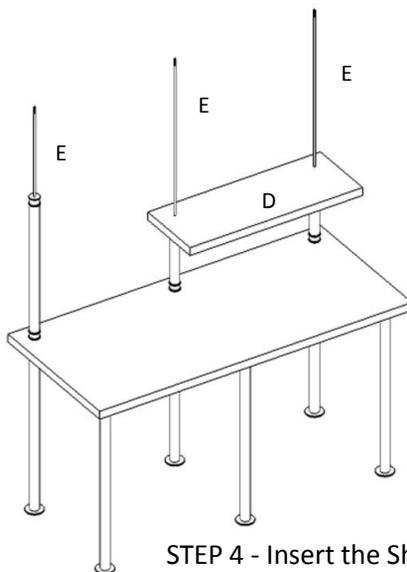
STEP 4 - Insert the Short shelf (D) onto Solid Rod (E) as shown above.
