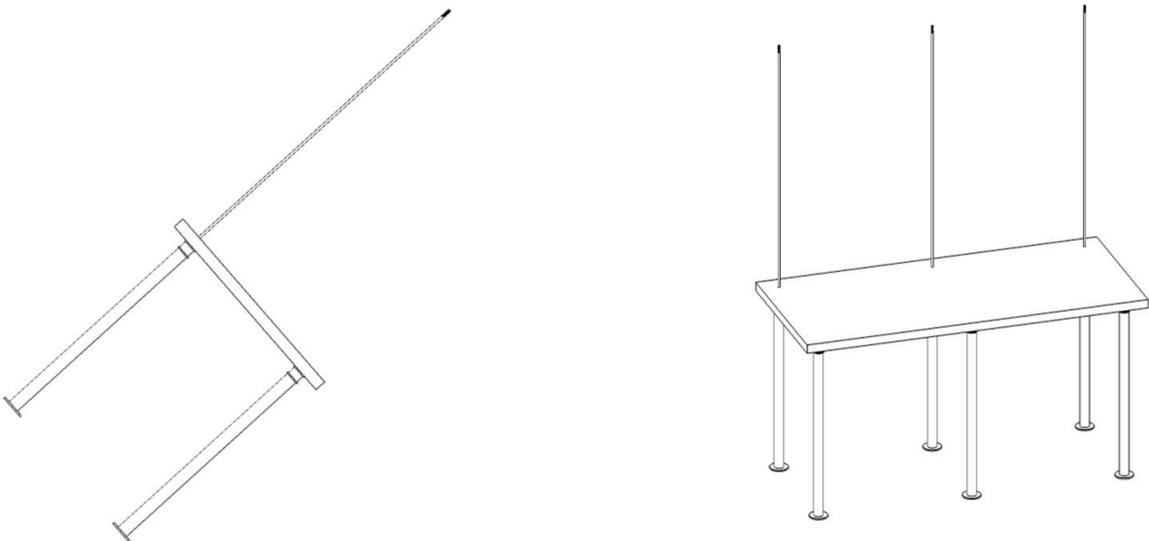
**STEP 2 - Insert combined Bottom Leg (F) & Solid Rod (E) pieces through Table Top (B) in predrilled locations. Base structure will be ready as shown above.**
