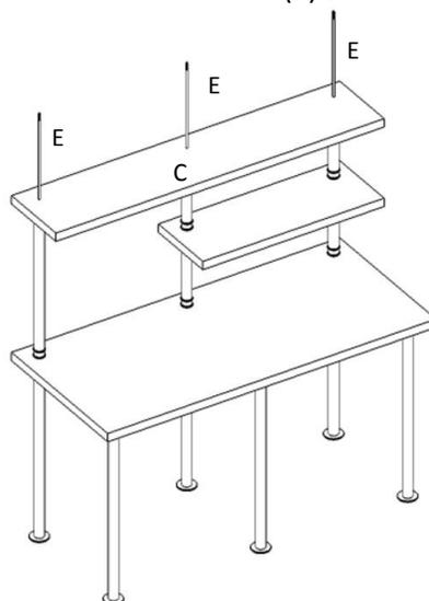
STEP 6 - Insert a Long Shelf (C) onto the Solid Rod (E) as shown above.
