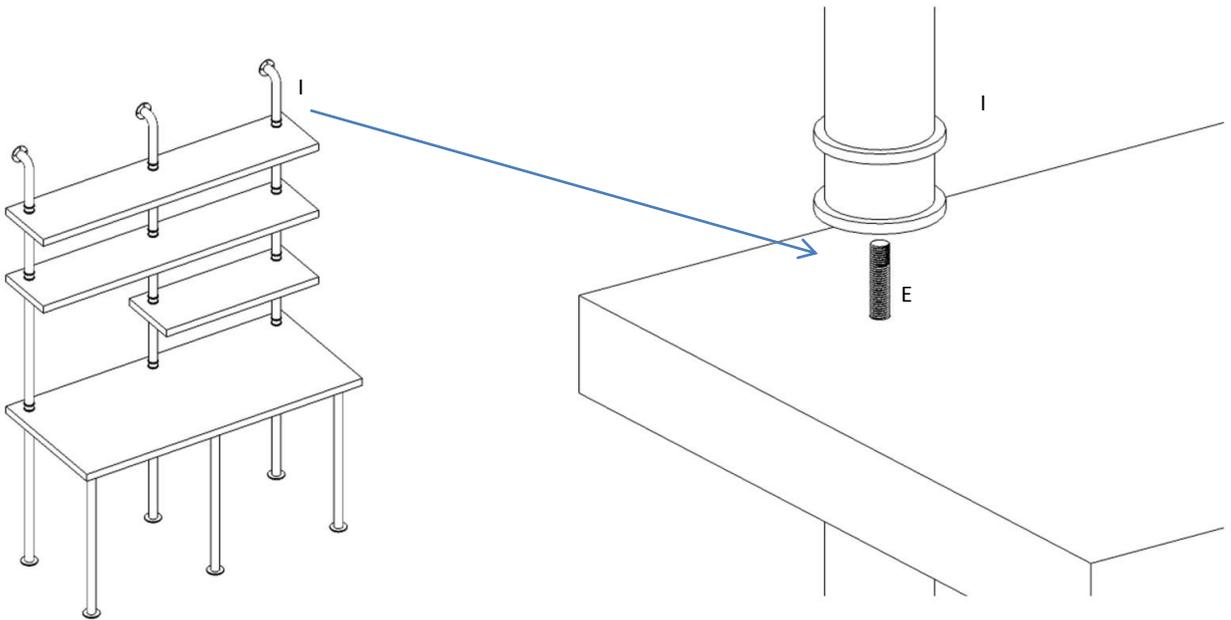
STEP 9 - Attach the Bent Pipe (I) to Solid Rods (E).
