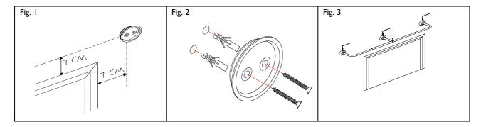
I M P O R T A N T: It is highly recommended that the brackets be attached to a structural wood support, such as molding around the window or wooden studs within the walls. If the studs within the wall are metal, you must pre-drill into the metal stud and use sheet-metal screws.
