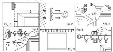
I M P O R T A N T: It is highly recommended that the brackets be attached to a structural wood support, such as molding around the window or wooden studs within the walls. If the studs within the wall are metal, you must pre-drill into the metal stud and use sheet-metal screws.
