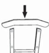
4-5. Lock both the side legs to the vertical frame tightly. Apply pressure when turning the screw into the drill hole. The screw and drill holes were engineered to be a close fit in order to provide stability.
