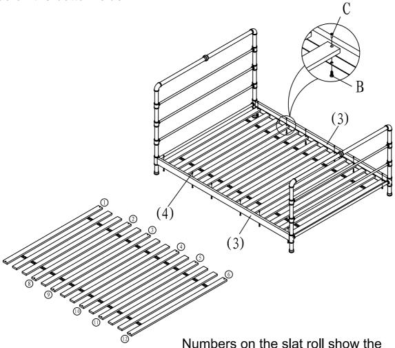
Numbers on the slat roll show the locations to tighten the bolts and nuts.
